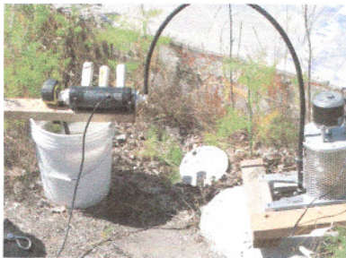
Flow cell in use with Rotapump™
